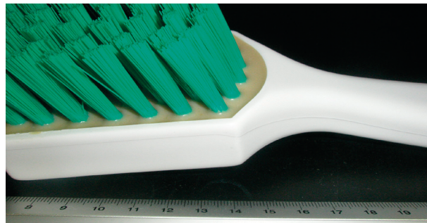
Figure 7a. Drilled and stapled resin set brush sample.
