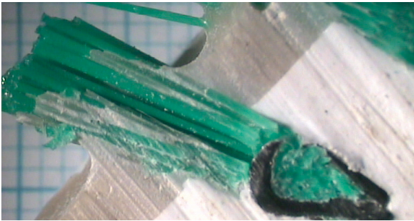
Figure 7d. Light microscope image of a vertical cross-section of a drilled and stapled resin set bristle bundle showing a potential contamination trap.
