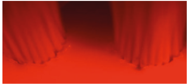
Figure 4b. Light microscope image of the area where the bristles enter the brush head.
