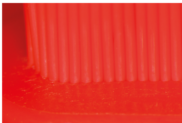
Figure 10b. Light microscope image of the area where the bristles enter the brush head.
