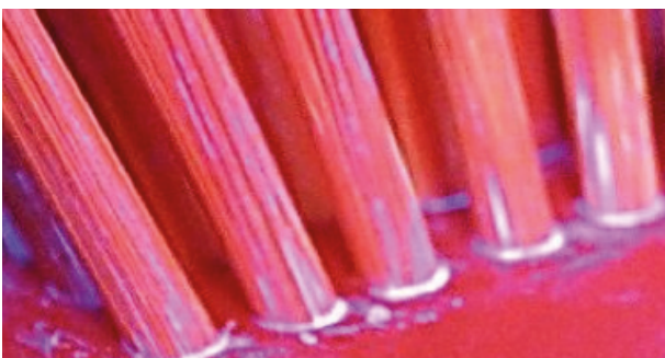
Figure 5a. Drilled and stapled brush after cleaning. UV lotion trapped in the drilled holes.
