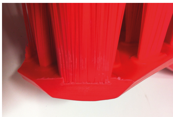
Figure 10d. Vertical cross-section through a UST bristle bundle showing its fully moulded construction.
