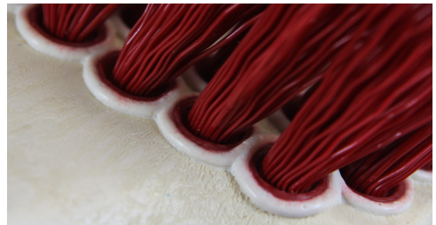
Figure 8b. Image of the area where the bristles enter the brush head.
