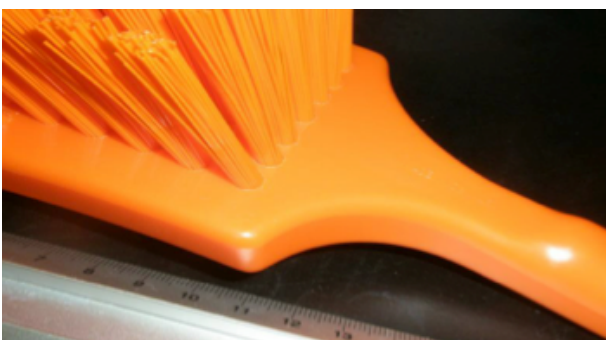
Figure 4a. Drilled and stapled brush sample.
