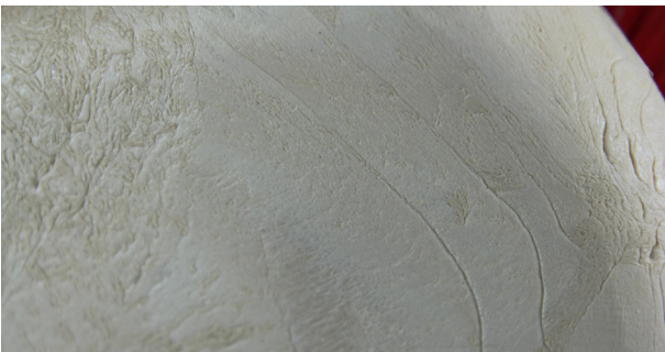
Figure 8d. Close up image of the surface of the fused bristle brush - potential contamination traps.
