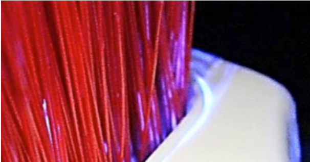
Figure 6c. UV lotion remaining on and in the brush block after brush cleaning.
