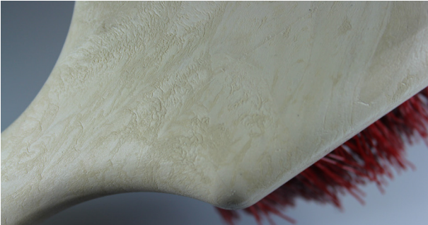
Figure 8c. Back of the fused bristle brush, poor surface finish.
