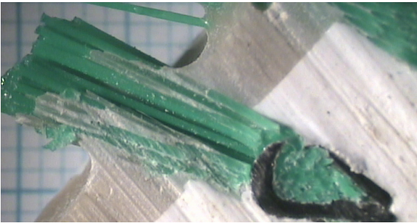
Figure 7d. Light microscope image of a vertical cross-section of a drilled and stapled resin set bristle bundle showing a potential contamination trap.
