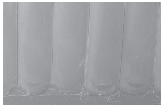
Figure 10c. Scanning electron microscope image of the area where the bristles enter the head of a UST brushware product.
