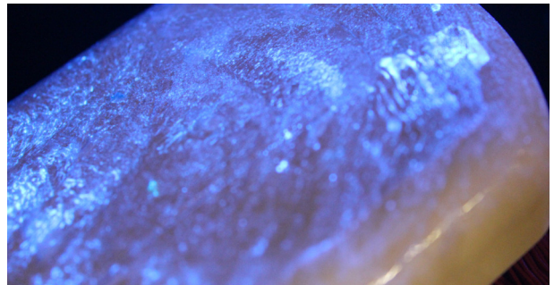
Figure 9b. UV lotion retained by the brush surface - poor surface finish.
