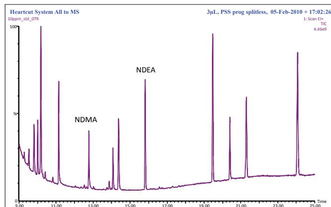
Figure 3. Total ion chromatogram ( $m/z$  35 to 150) from a 3 μL injection of a 10 ppm standard mixture of nitrosamines with the precolumn effluent directed to the second column and the MS detector.
