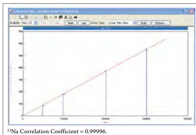
Figure 2. Calibration curve for <sup>23</sup>Na (0-300 ppm).
