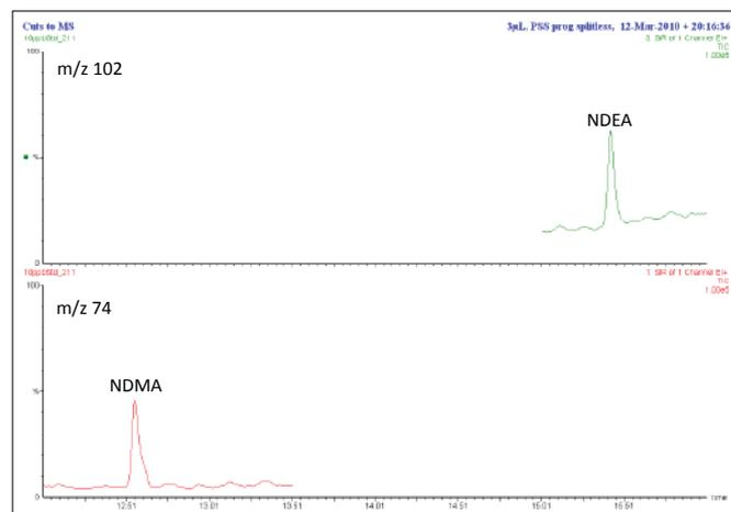
Figure 7. SIR chromatographic traces at  $m/z$  74 and 102 showing expected elution times of NDMA and NDEA respectively from an injection of a 10 ppb stand mixture of nitrosamines (equivalent to 1 ppb in samples).
