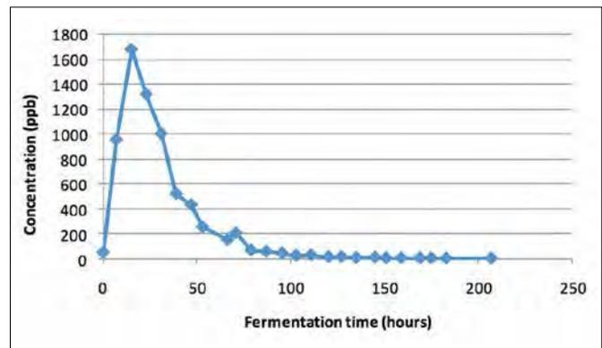
Figure 10. Concentration profile of 2,3-butanedione for the experimental beer during the fermentation process.
