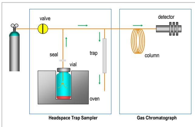
Figure 3. Schematic diagram of the HS trap system showing the pressurized headspace being released from the vial into the adsorbent trap.
