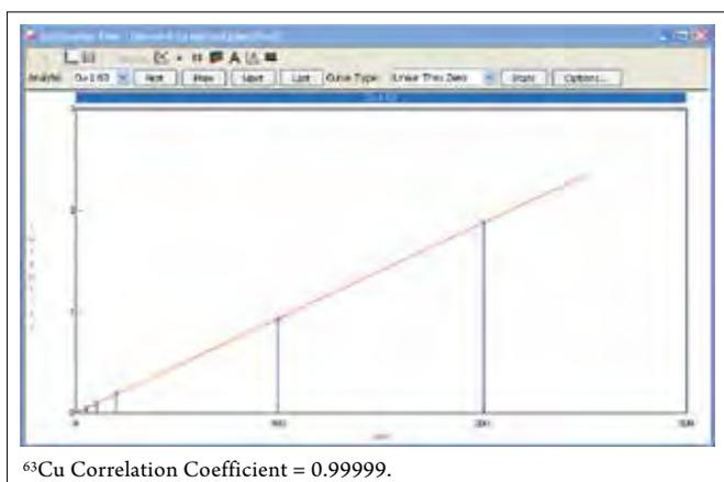
Figure 3. Calibration curve for <sup>63</sup>Cu (0-200 ppb).
