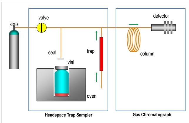
Figure 4. Schematic diagram of the HS trap system showing the VOCs collected in the adsorbent trap being thermally desorbed and introduced into the GC column.
