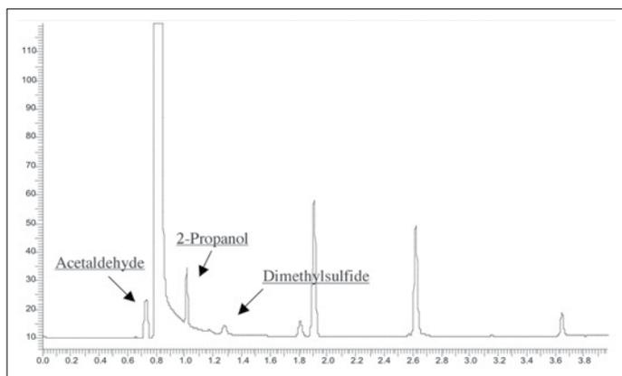
Figure 3. Acetaldehyde determination at 10-ppm concentration (FID).
