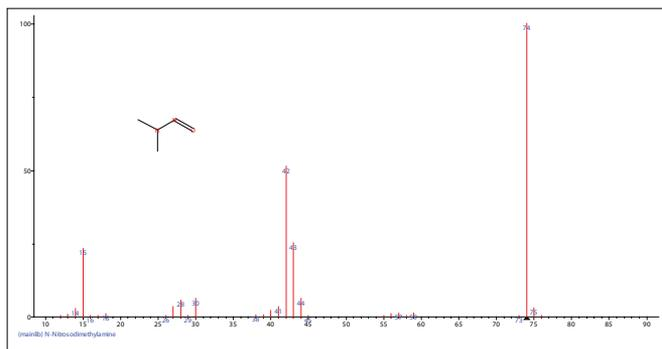
Figure 5. Structure and mass spectrum of nitrosodimethylamine.
