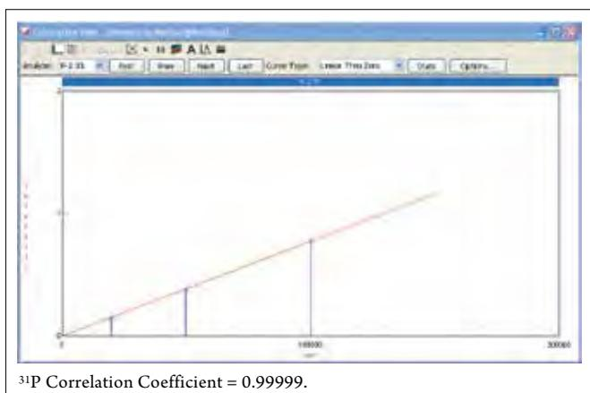
Figure 4. Calibration curve for <sup>31</sup>P (0-100 ppm).
