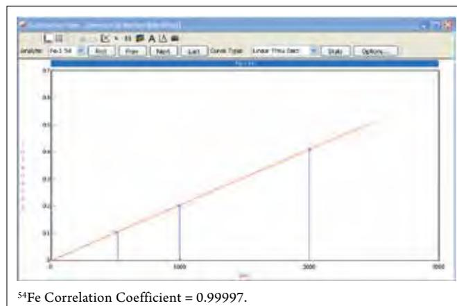
Figure 1. Calibration curves for <sup>54</sup>Fe (0-2 ppm).
