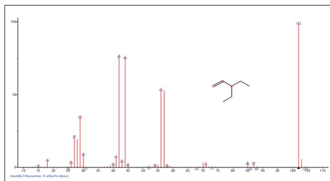
Figure 6. Structure and mass spectrum of nitrosodiethylamine.
