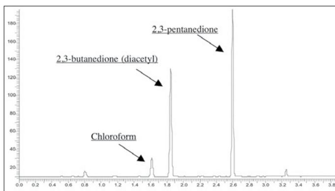
Figure 2. Vicinal diketones determination at 10-ppb concentration (ECD).
