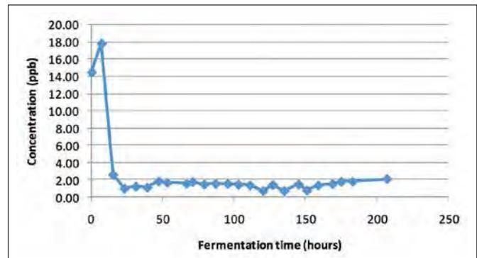
Figure 11. Concentration profile of dimethyl sulfide for the experimental beer during the fermentation process.
