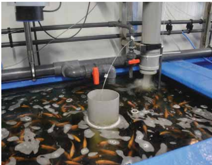
In aquaculture the wastewater is directly recirculated back into the fish tanks. In Aquaponics there is a double recirculation system, so optimum conditions can be set up independently
