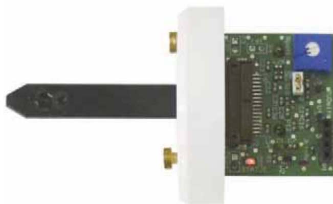
Figure 6: The prototype sensor which can be inserted into the carcass (left black piece, right processing unit covered with container during operation), and records temperature and pH during the processing in the slaughterhouse
