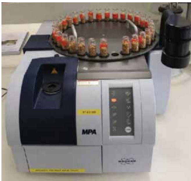
Figure 1: NIR instrument equipped with a wheel of 30 sample holders (Bruker MPA)
