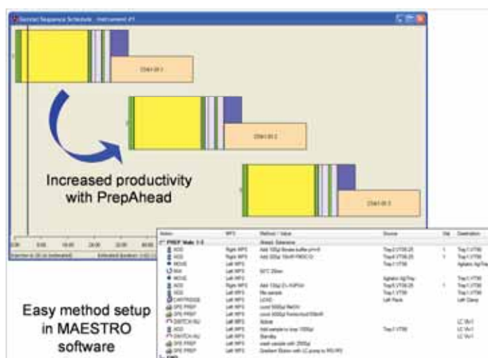
Figure 3a. Sequence of scheduled events in the Maestro software for online SPE: green - adding buffer and FMOCl, yellow - derivatization, light blue - online SPE, orange LC-MS/MS analysis, dark blue washing of the autosampler, the PrepAhead function increases productivity by simultaneously preparing the following sample while perming LC-MS/MS analysis of the previous sample
