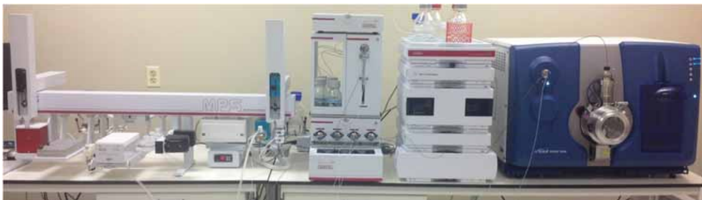
Figure 2. GERSTEL MPS 2XL with SPE XOS coupled to an QTRAP ® 4500 system
